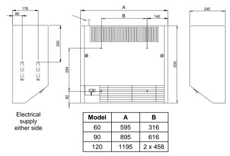
3 Connect the heating system flow and return pipes to the heater pipe work. Do not use soldered fittings to the heater pipe work as the heat generated may cause damage to internal wiring and components.
