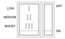
It is recommended that the model chosen is capable of maintaining the calculated heat loss at medium heat output enabling the boost setting to be used for faster heat up and the low speed for maintaining temperature.
